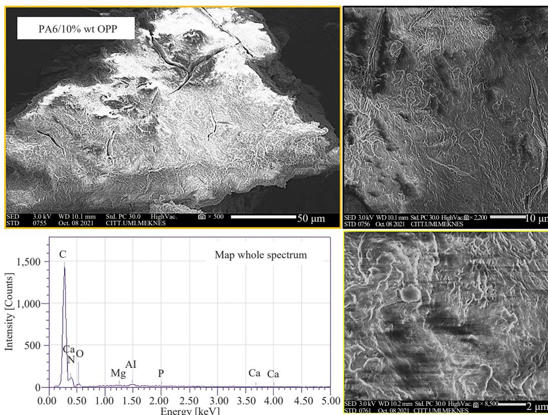
Figure 6. SEM image of the surface of a PA6/OPP pellet without contact with bacteria
