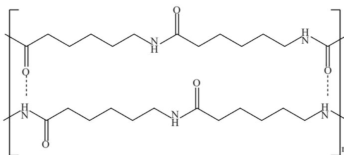
Figure 1. Hydrogen bonding between molecular chains of PA6
